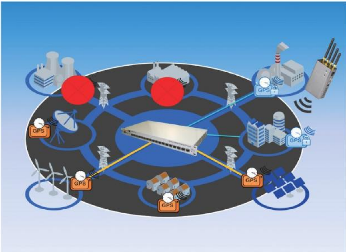
WR Switch backup for Jammed GPS signals.
