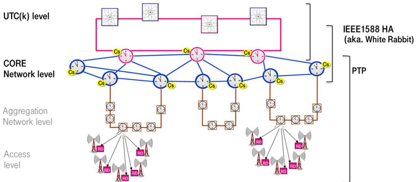
Figure 1: Backbone distributed topology - Source: Deutsche Telekom
