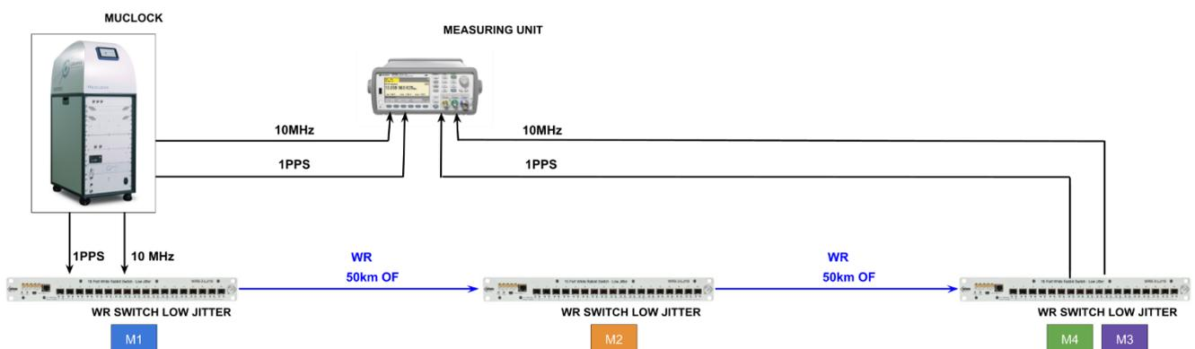
**Figure 1: Test set-up**
