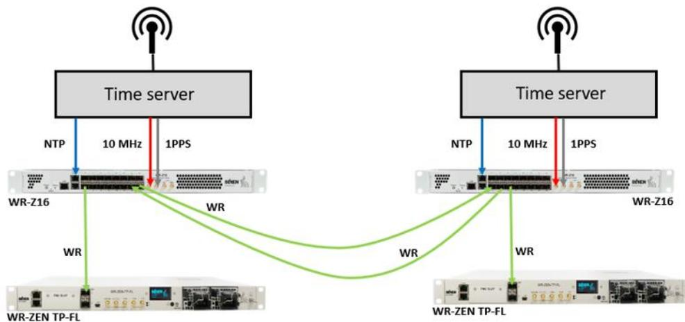
**Figure 2: Example of the resilience GNSS link for 2 locations.**
