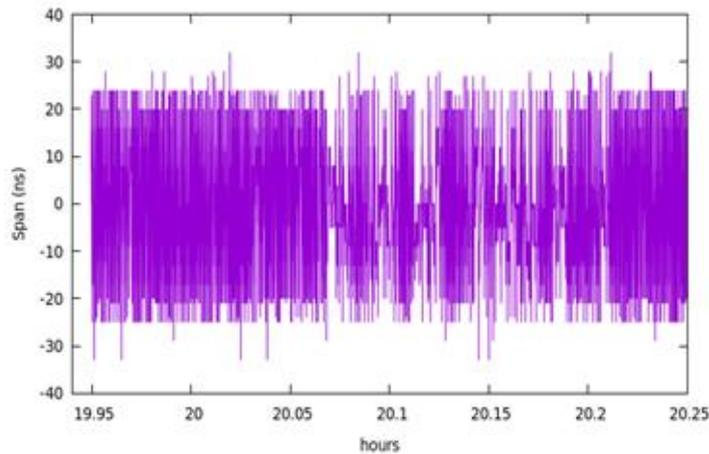
Figure 3. Time Synchronization Accuracy
