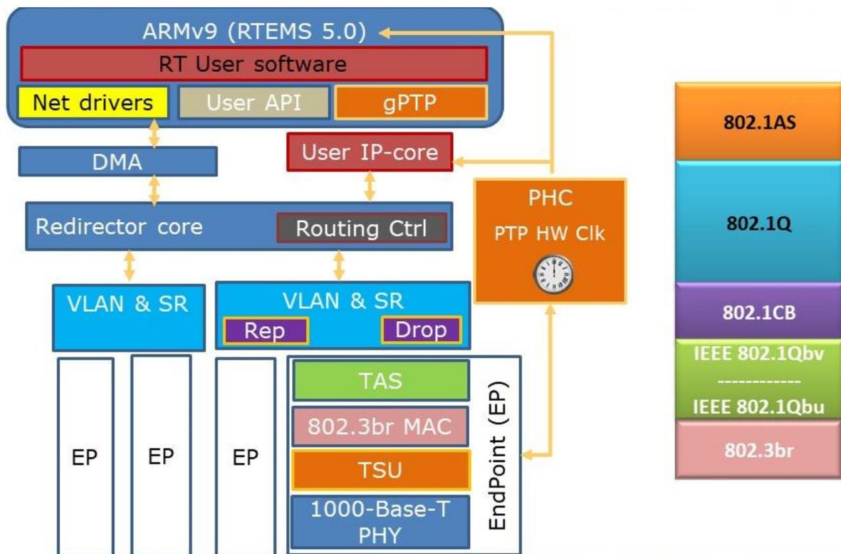
Figure 1. Architecture of the Giga Ethernet Light TSN Bridge
