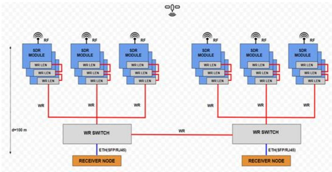
Figure 3. ULF antennas synchronization example
