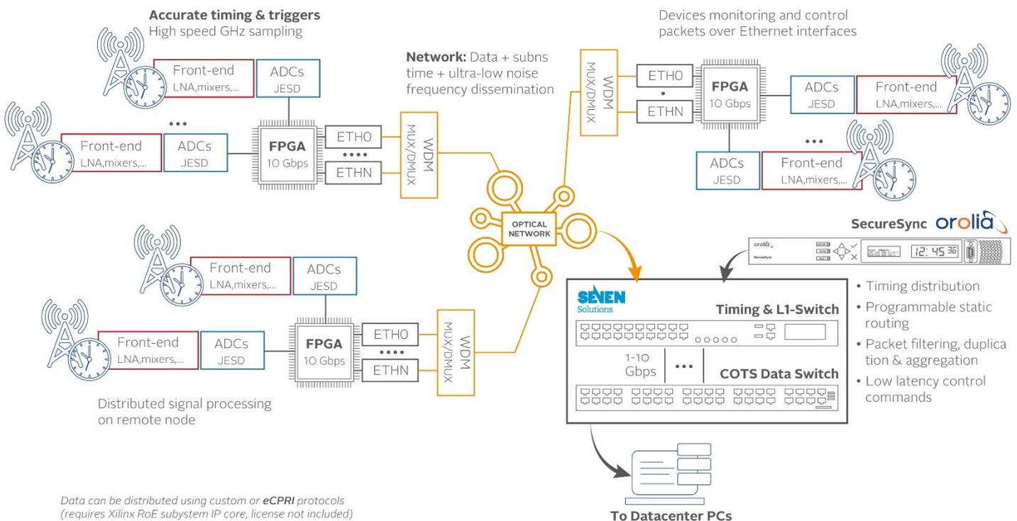
Figure 1. Example of RoE utilization for distributed communication ground segment facility
