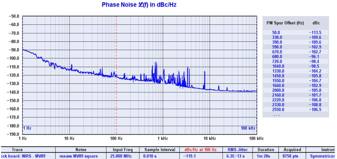
Figure 2. Phase noise of a 25MHz signal distributed over 5 Km of fiber using Seven Solutions White-Rabbit technology
